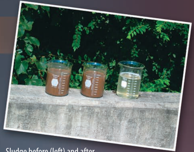
Sludge before (left) and after (right) treatment with Geotube® dewatering technology
