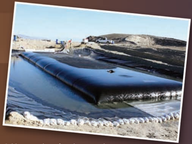
Gold mine tailings from barren and pregnant ponds dewatering in Geotube® containers
