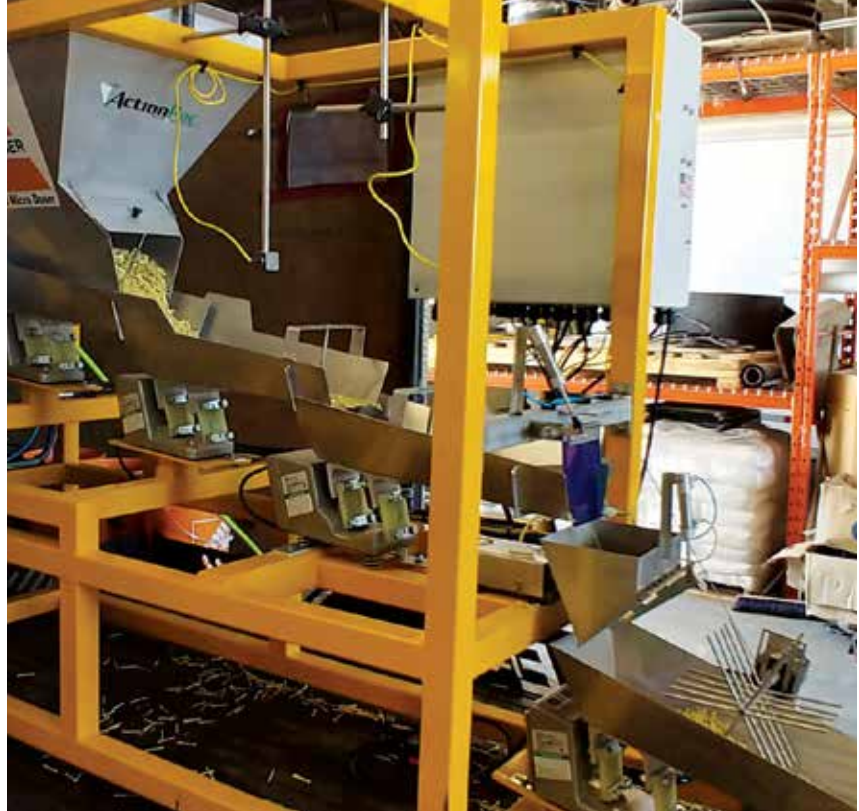
The Micro Doser MD3.0 delivers ACE Fiber™ continuously to either the Drum or Pug Mill
