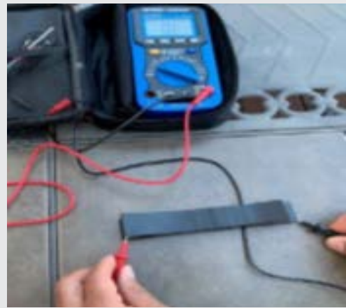
Figure 3. Using ohmmeter to qualify conductive side
