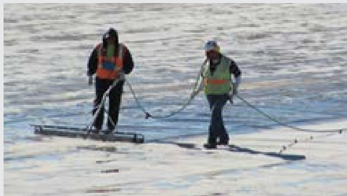
Figure 4. Water Puddle Testing
