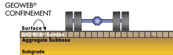
**As a surface stabilization system,** the GEOWEB® structure distributes surface pressures for dynamic and static loading, **controlling rutting and reducing long-term maintenance requirements and costs.** Using permeable infill with a high porosity, the system offers environmental and stormwater management benefits.
