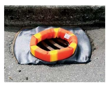
Catch basin donuts (CBDs) are an inlet control device installed on top of a catch basin to collect silt and sediment while letting the water pass through freely. Layfield's CBDs prevent water pooling during heavy rainfalls and allow for a much higher flow rate.
