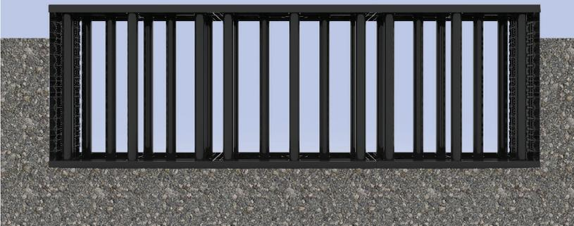
*Modules are to be backfilled evenly in 12" (305mm) lifts.*
