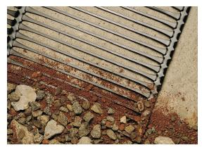
A high-density polyethylene, homogeneous product that does not require weaving, coating or welding to maintain the product's integrity.
