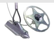
Falcon Anchors™ can be used to create erosion control systems designed to firmly secure and support soils deep into the soil strata. These are used for permanent installations utilizing our TRM and HPTRMs. A drive rod and jackjaw assembly required for proper installation.
