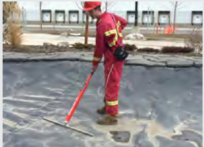
Figure 5. Arc Testing on an exposed geomembrane
