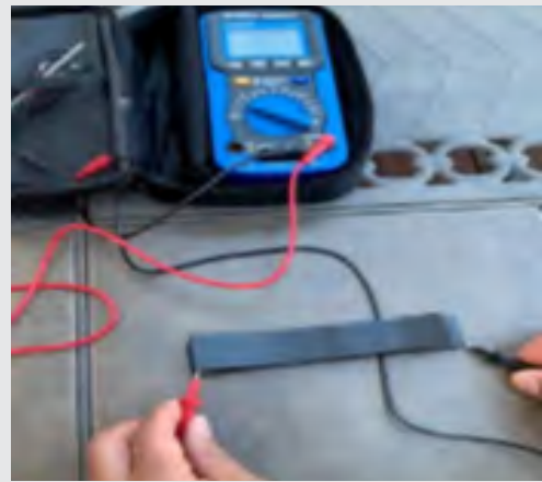
Figure 3. Using ohmmeter to qualify conductive side
