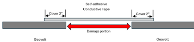
Figure 5: Illustration of covering the damage area.
