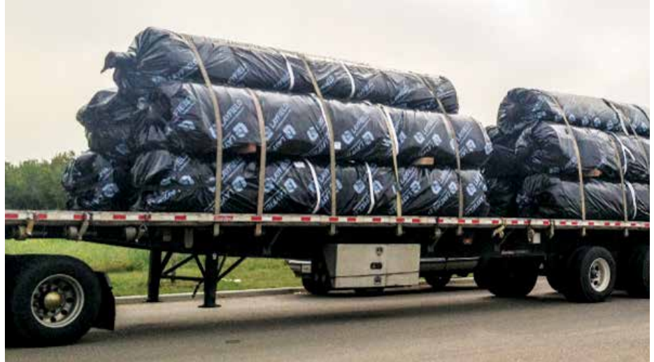
Figure 11. Layfield truck carrying prefabricated geomembranes for delivery
